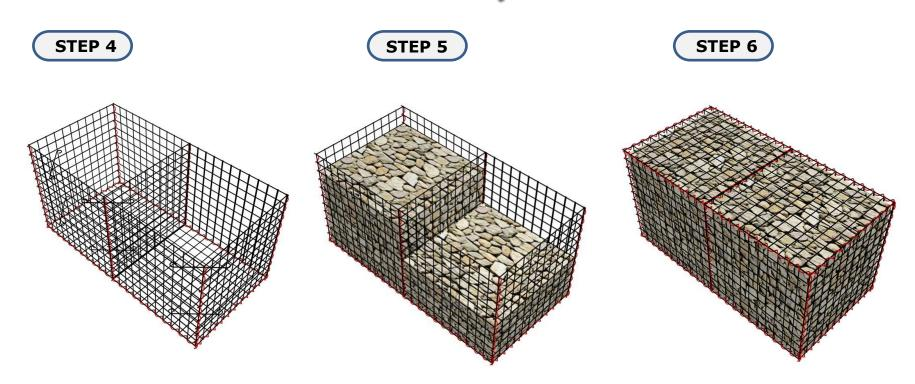
18" Corner Stiffeners should be placed inside at 12" intervals(4 per cell) and crimped over the line and crosswire on the front and side faces. None are needed for interior cells. Lacing wire may be used as an alternate cell cross tie in lieu of Corner Stiffeners, tying from front to back at 12" intervals.
