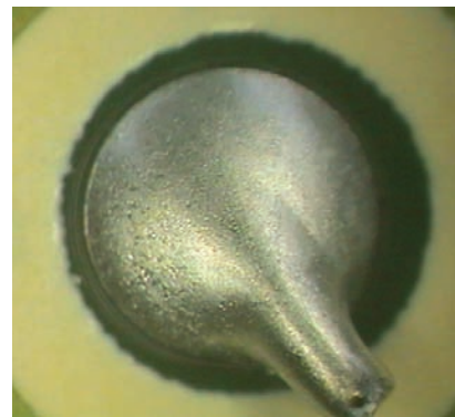
After using Shrinkage killer Solder
